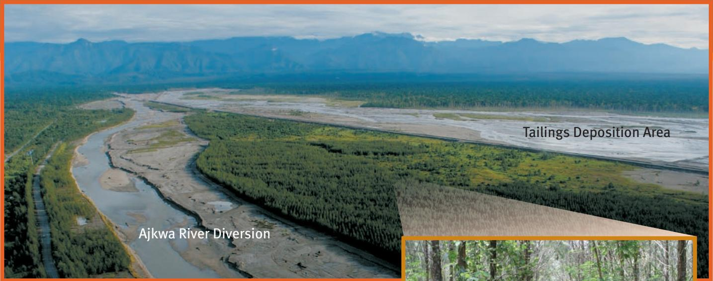
*Work was completed to divert the Ajkwa River out of the tailings deposition area (above right) and into its historic channel (above left). Re-directing the Ajkwa in this manner decreases the amount of water entering the tailings management area. The tailings in the foreground of the picture were deposited before the diversion and are being reclaimed.*
